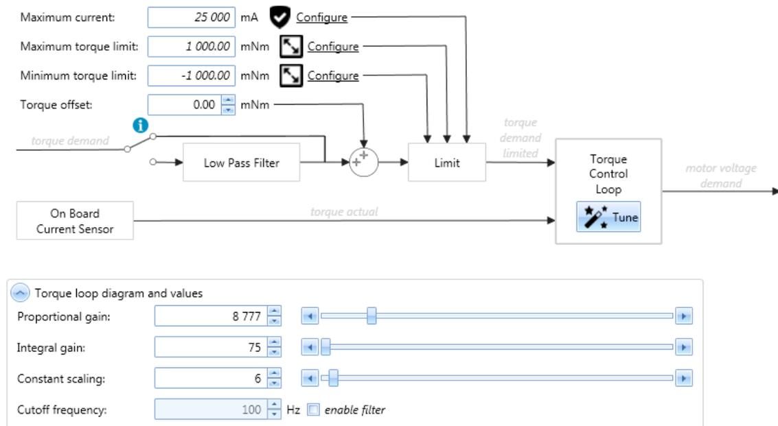
**Max current** parameter indicates the maximum permissible current creating torque in the motor.
