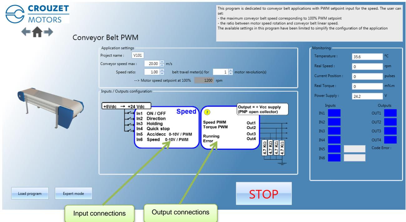
The "Conveyor Belt PWM" application program invokes the V101 expert program. The user can switch to this expert mode at any time to access all the settings by clicking the "Expert Mode" button.
