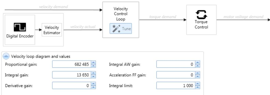
Note that you can set the position loop (or alternatively the velocity loop) for velocity modes such as homing or profile velocity with a selector:
