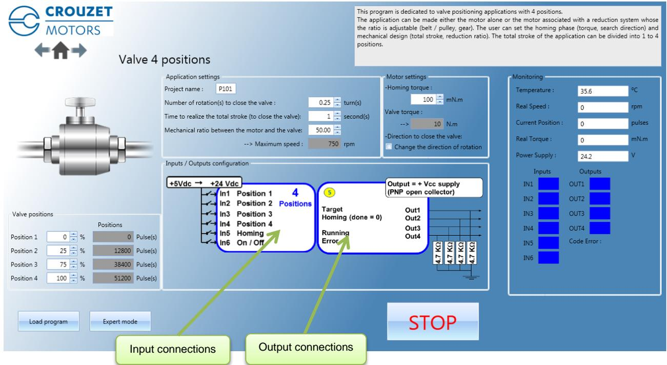
The "Valve 4 positions" application program invokes the P101 expert program. The user can switch to this expert mode at any time to access all the settings by clicking the "Expert Mode" button.
