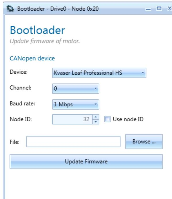
Select the .hex file that you want to load inside the SMI21 CANopen drive by click on the “Browse” button and after click on the “Update Firmware” button to launch the bootloader sequence.
