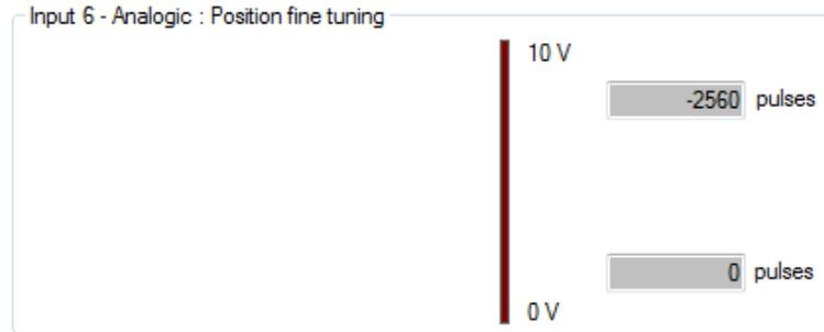
The motor position setpoint is the addition of position setpoint of IN5 and of position setpoint of IN6.
