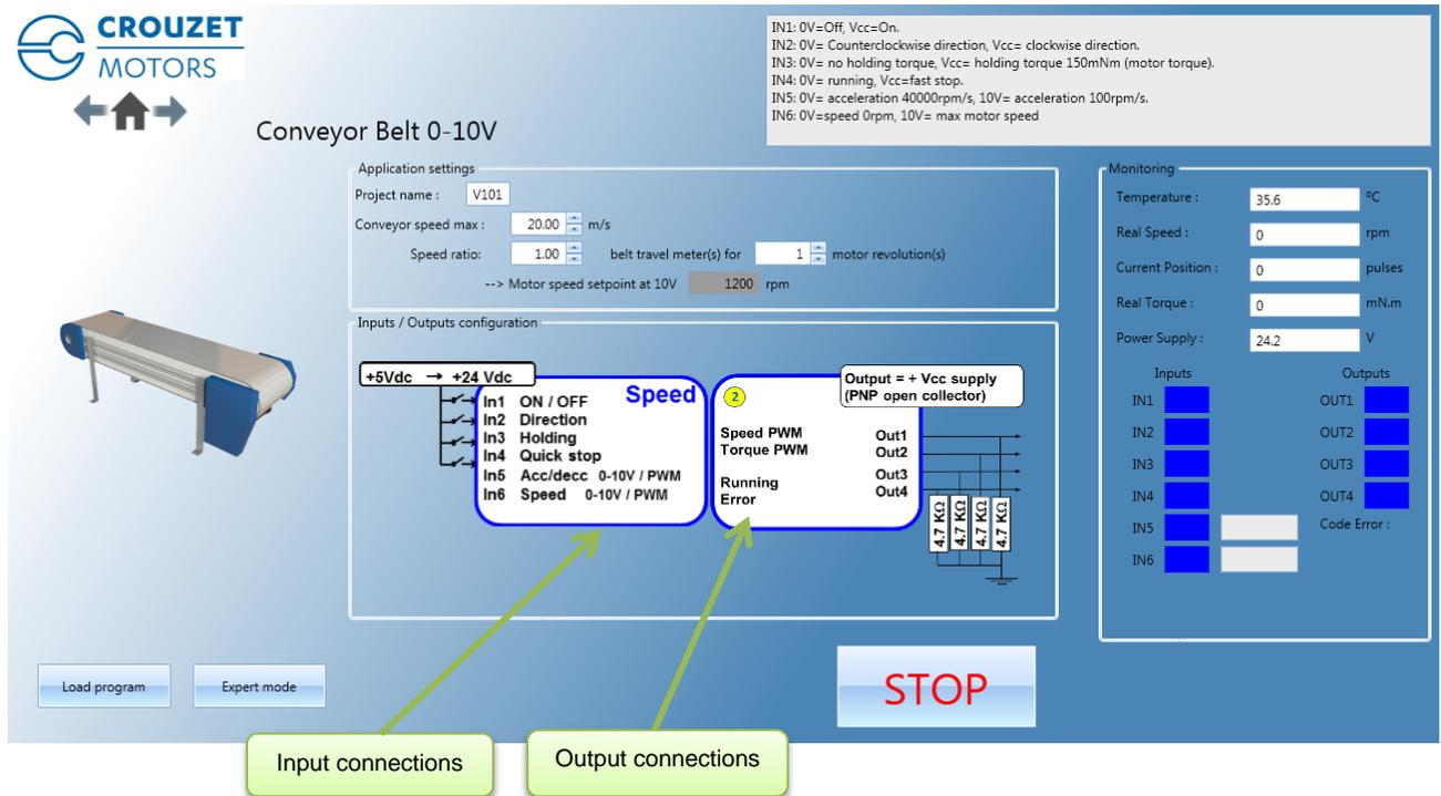
The "Conveyor Belt 0-10V" application program invokes the V101 expert program. The user can switch to this expert mode at any time to access all the settings by clicking the "Expert Mode" button.
