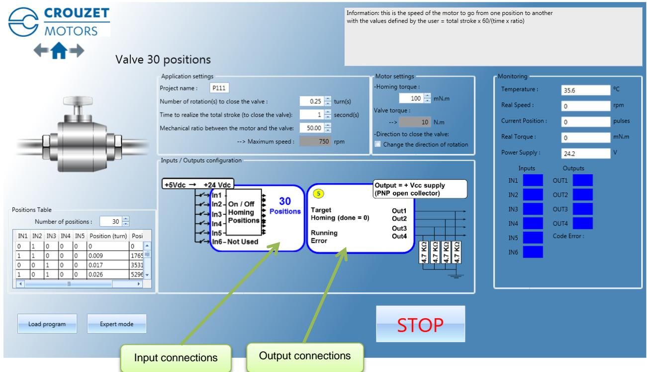
Information: this is the speed of the motor to go from one position to another with the values defined by the user = total stroke x 60/(time x ratio)
